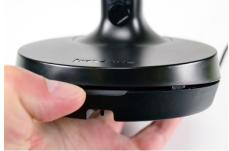
If installing a peripheral cable, lift the top cover from the base using the small lip above the LED on the front of the base.
