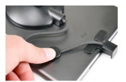
42 Adjust the position of the cable to tighten any slack and place the cable manager over the cable. Apply pressure for at least 10 seconds.
