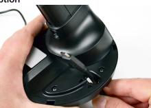
Insert the USB-C end of the cable up through the hole in the base.
