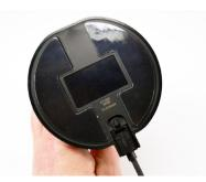
35 Plug the CT3012 power connector into the CT1503 handle.
