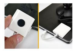
50 **Optional:** A small piece of adhesive can be placed on the adapter to keep it secured to the back of the tablet.
