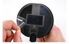
46 Peel the clear film from the 2 adhesives on the handle.
