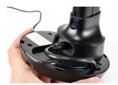
Plug the cable into the port in the base.
