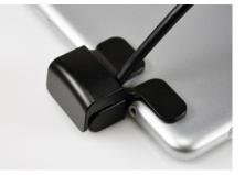
Place the procetive cap over the power connector, with the adhesives on the back of the tablet. Apply pressure for at least 10 seconds.
