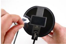
26 Peel the clear film from the 2 adhesives on the handle.
