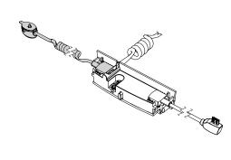
Choose correct size anti-rotation bracket and place into groove in sensor. Slide sensor together to confirm bracket is up against back of camera. Tighten screws with T-20 bit.
