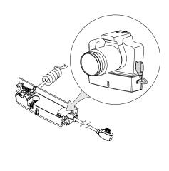
Optional: Plug lens sensor into camera port (opposite power connector).
