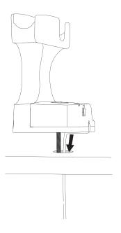
Firmly press stand to fixture for at least 10 seconds. Below counter, attach washer to one threaded screw. Twist wing nuts to tighten both screws.
