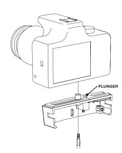
Plug power connector into sensor port closest to camera power plug. Note: There are 2 ports power connector can be plugged into.
