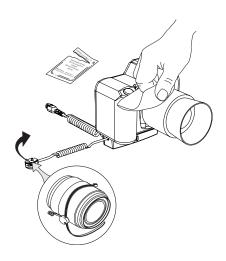
Place sensor into stand. Plug sensor into alarm unit.
