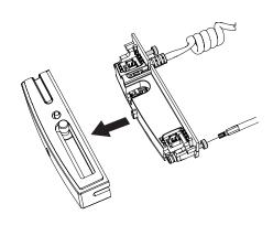
Attach camera to sensor. Center and tighten screw with T-20 bit. Confirm plunger is completely depressed.
