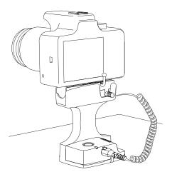
**To arm/disarm:** Place IR key onto IR lens on alarm unit. Press button once to arm or disarm system.
