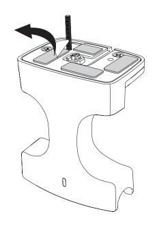
h Route threaded screw and power cord through hole in fixture.
