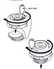
Turn key fob clockwise to reel in cord. inches of cable between housing and
